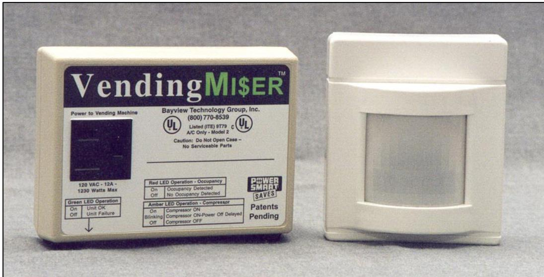
A vending miser consist of a motion sensor and the miser itself (see picture). The vending machine is plugged into the vending miser, which is attached to a wall and plugged in to an outlet. The motion sensor is plugged in to the vending miser.
