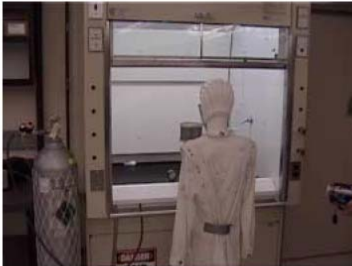
Tracer gas test being performed on the Air Sentry fume hood
