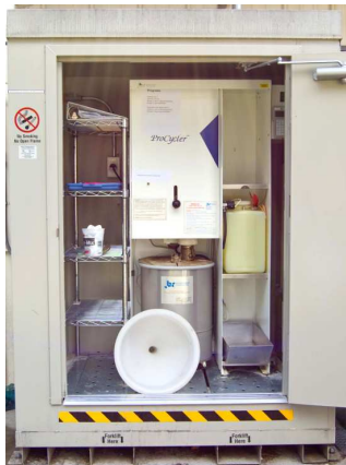
Distillation unit in explosion-proof enclosure
